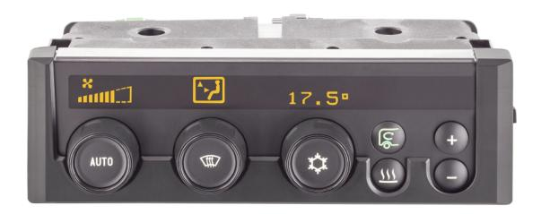
All functions of an air conditioner can be controlled using the ACCU plus. All settings, such as the interior temperature, auxiliary heating or blower speed, are easy to read from the clearly arranged LC display. Its compact design allows the ACCU plus to be integrated easily into any dashboard.
