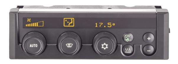
All functions of an air conditioner can be controlled using the Climate operating panel. All settings, such as the interior temperature, auxiliary heating or blower speed, are easy to read from the clearly arranged LC display. Its compact design allows the COP to be integrated easily into any dashboard.
