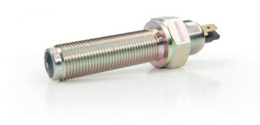
Inductive sensors are used in vehicles and machines to measure the revolutions per minute of rotating shafts, axles or wheels. The number of teeth of a toothed pulley or the holes of a holed pulley are counted by induction. The produced pulses will be transmitted to a revolution counter which will show the revolutions per minute taking into account the pulses per revolution.
