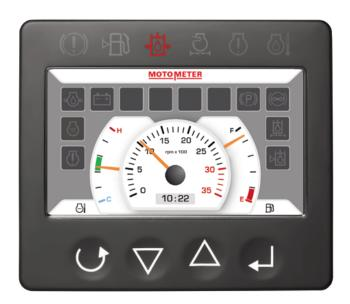
MCA 430 is a configurable multifunctional display and enables graphical presentation of different datas on the free designable, high-resolution 4,3" TFT colour display.
