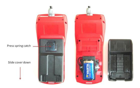
Press the spring catch on the battery cover at the back of the MOTOMETER ECT 700 Handset.
