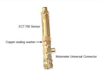
Connect the Sensor/MOTOMETER Universal Connector assembly to the MOTOMETER ECT 700
